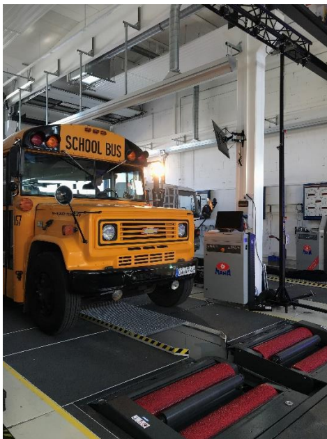
The yellow US school bus on the new digital CONNECT TRUCK brake tester.
