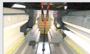
Ground anchor For holding the vehicle frame or the axle during lifting.
