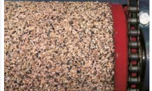
Plastic-coated roller surface VZ 935110
