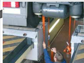
Hydraulic weight simulator VZ 935033
