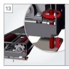
Continuously adjustable installation height (245-300 mm) of car floor assembly in the foundation or raised installation possible (patent pending).
