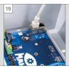
Two network/data interfaces, e.g. for ASA Livestream, internet link-in, network printers.
