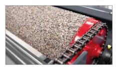
Roller surface plastic/granulate coated
