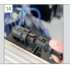
Easy plug-in connection of the CAN data bus (four wire) and drive motors.
