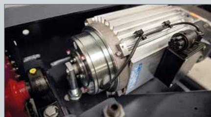
Electromechanical motor brake
