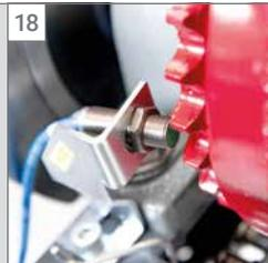
18 Best possible tyre-saving thanks to "real" slip monitoring by electronic sensor technology.
