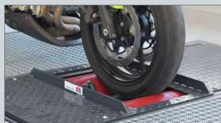
Roller set cover for motorcycle brake testing
