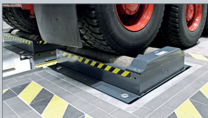
Roller set lift, hydraulic
