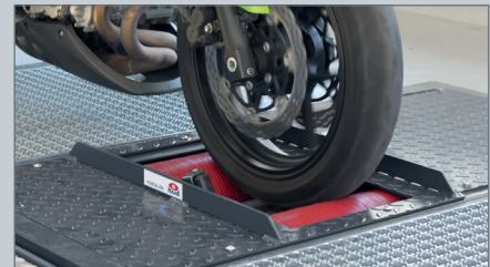
Roller set cover for motorcycle brake testing
