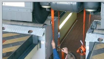
Pull-down device, hydraulic
