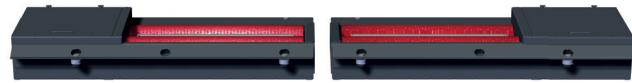
Digital roller brake tester C_MBT S 18.0 R160 MS with two-part roller set, up to 18.0 t axle load and a roller length of 1600 mm, motor positioned at the side of the roller set.
