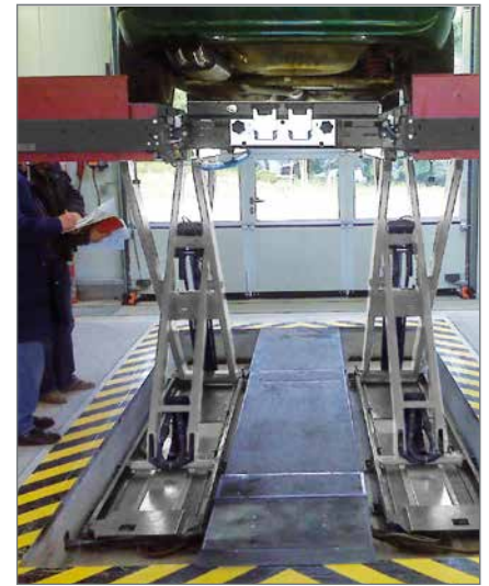
Centre platform facilitates an effective lifting height of 1850 mm.
