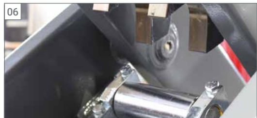
The cylinder raising support with step lever and rollers conducts a pure rolling movement. No sliding movement between the moving parts, meaning it is low noise, wear resistant and nearly maintenance-free.
