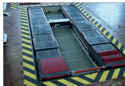
DUO CM in rectangular foundation with (optional) grating, (equipped for vehicle inspection test).
