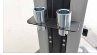
Sheet metal tray for support disc extensions.
